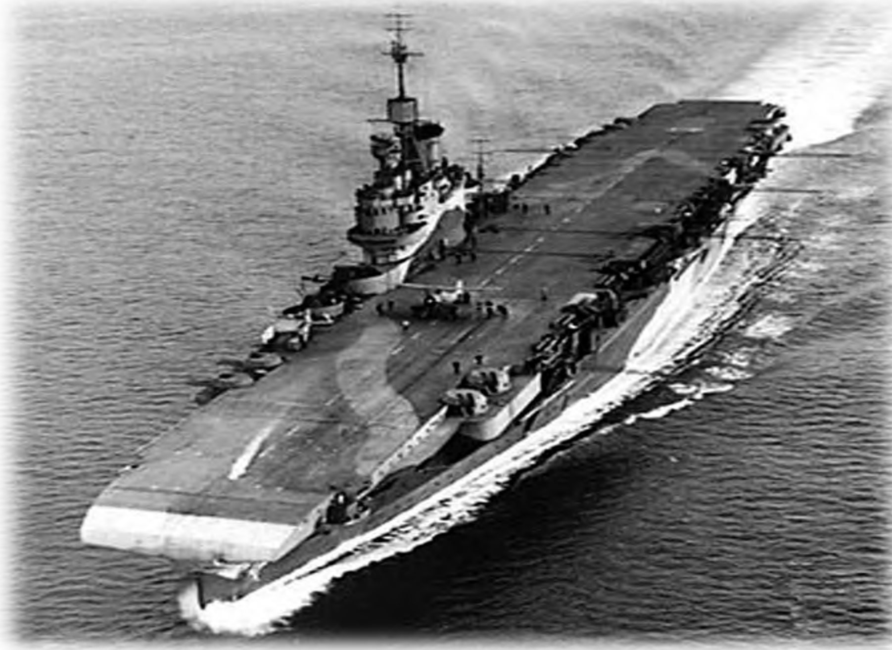
HMS Illustrious: 22,000 Tons, 740'(225.6m) long, 95'9"(29.2m) beam, top speed 30 knots
