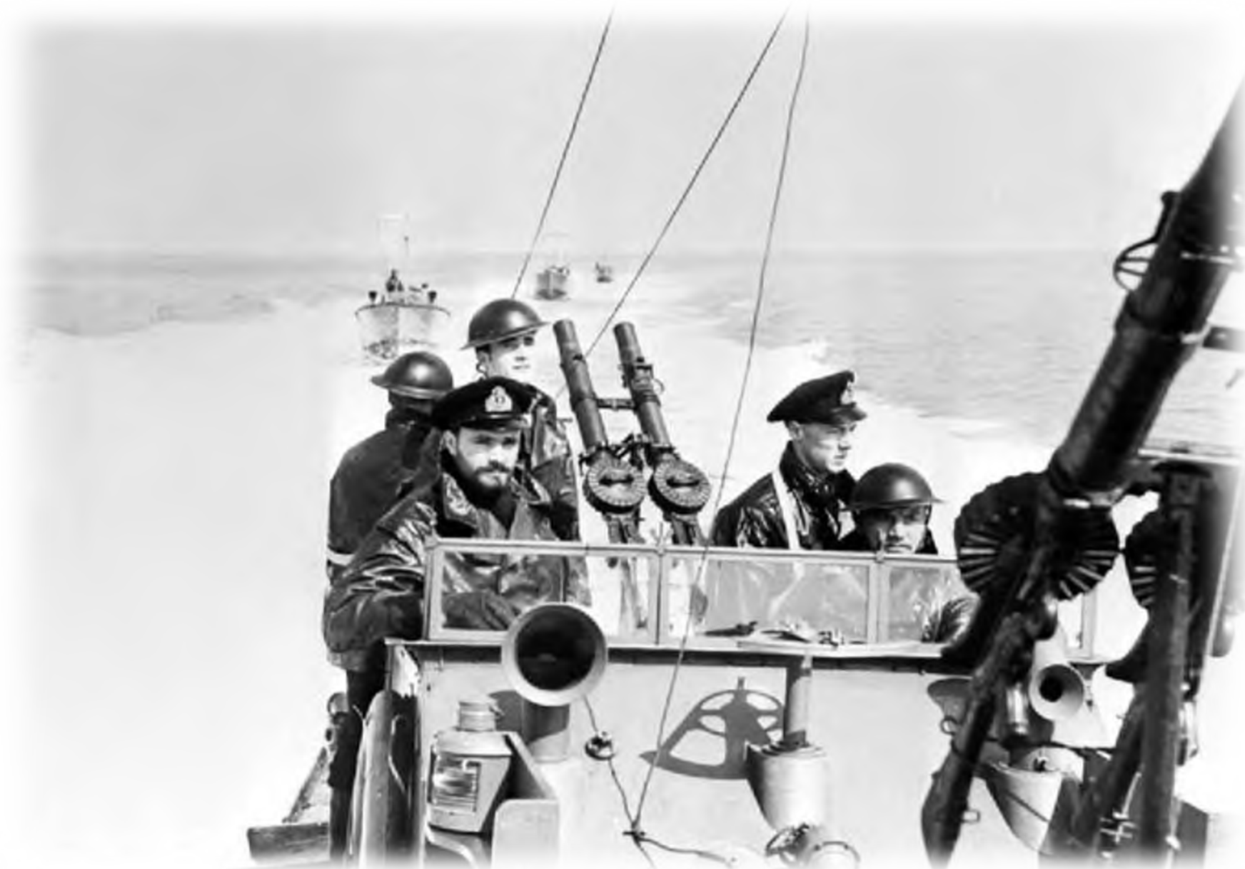
Twin-mounted Lewis Guns on a motor torpedo boat
