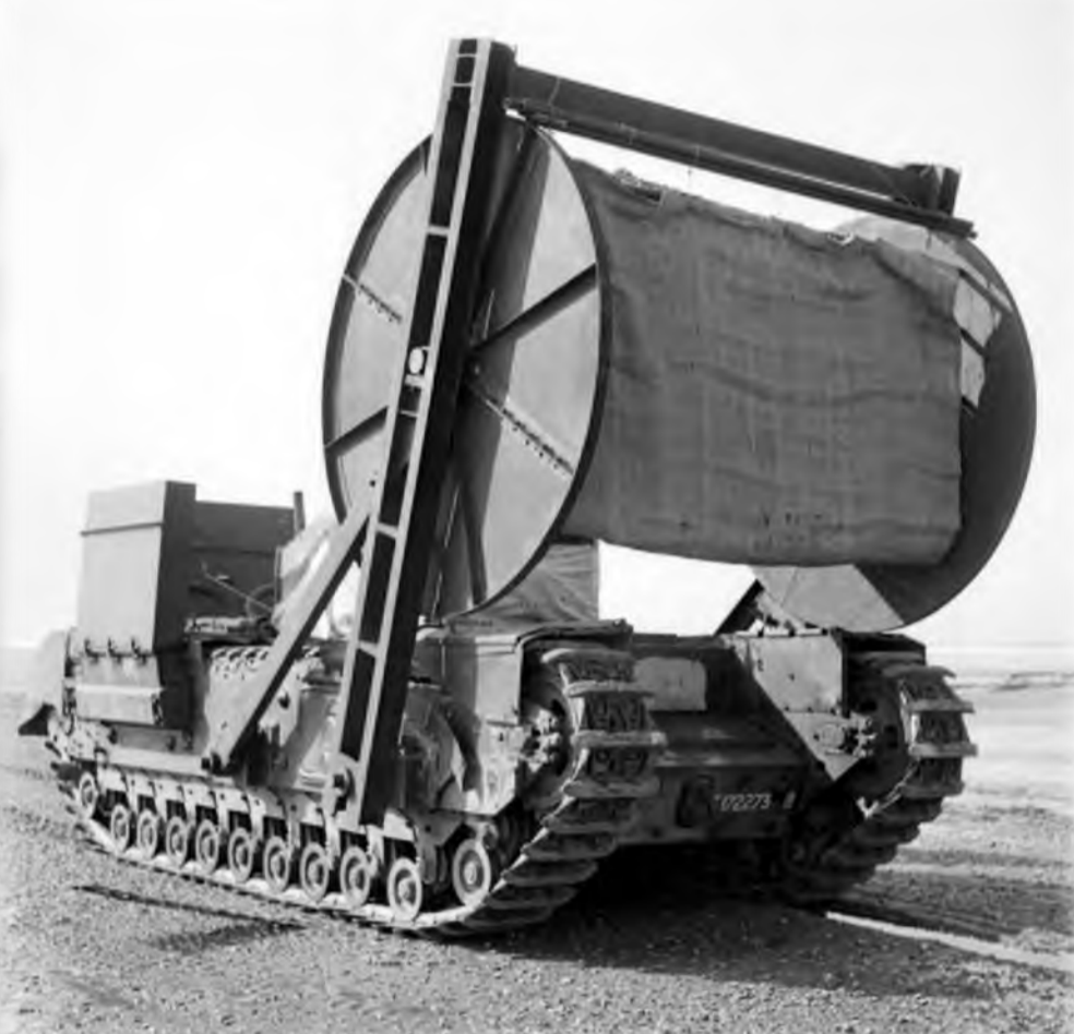
A Bobbin tank to lay a canvas track over soft ground.
