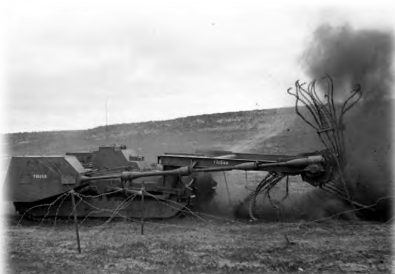
Mine Flail to clear a path through minefields
