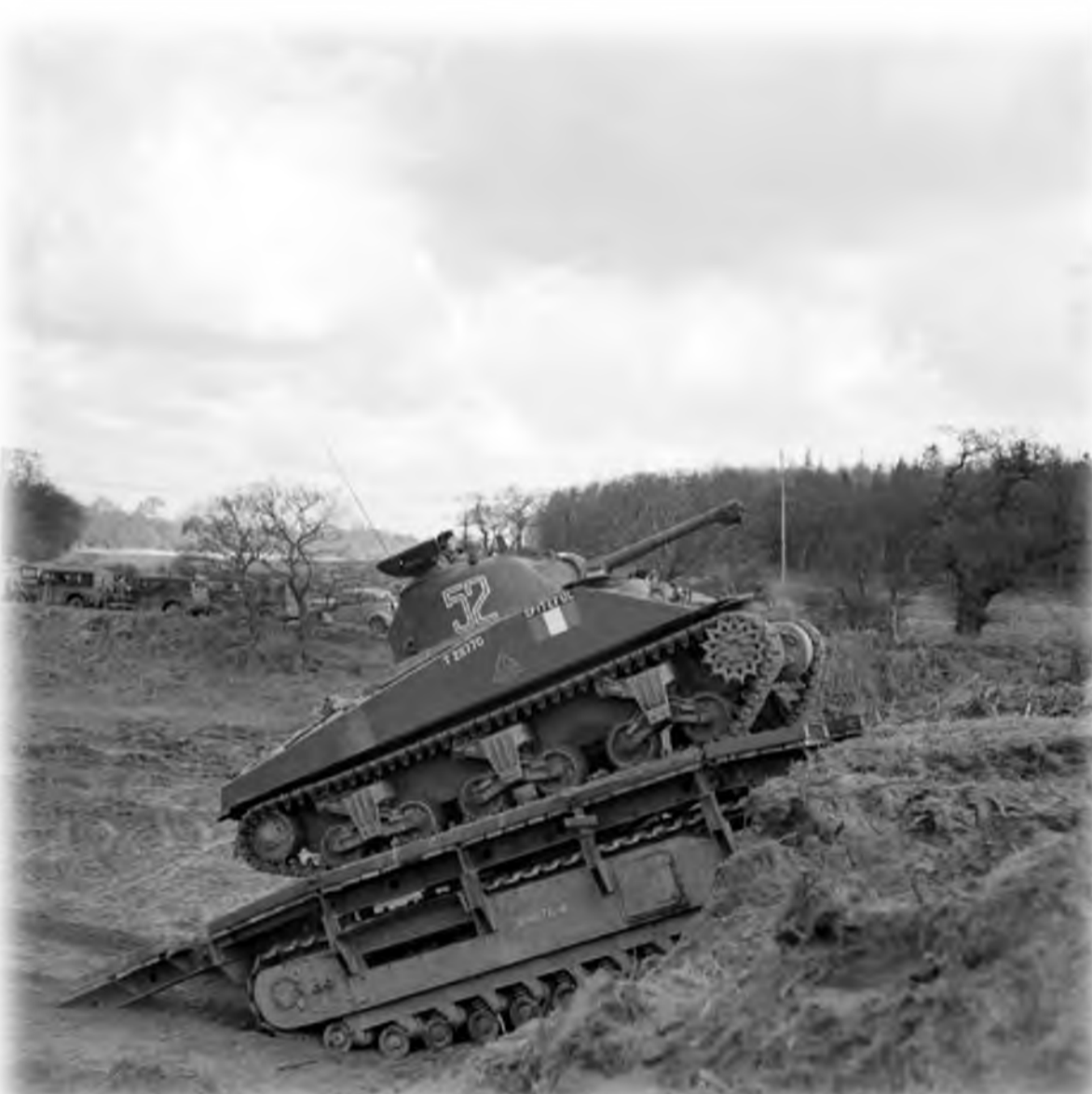
Sherman tank using an Armoured Ramp Carrier to scale obstacles
